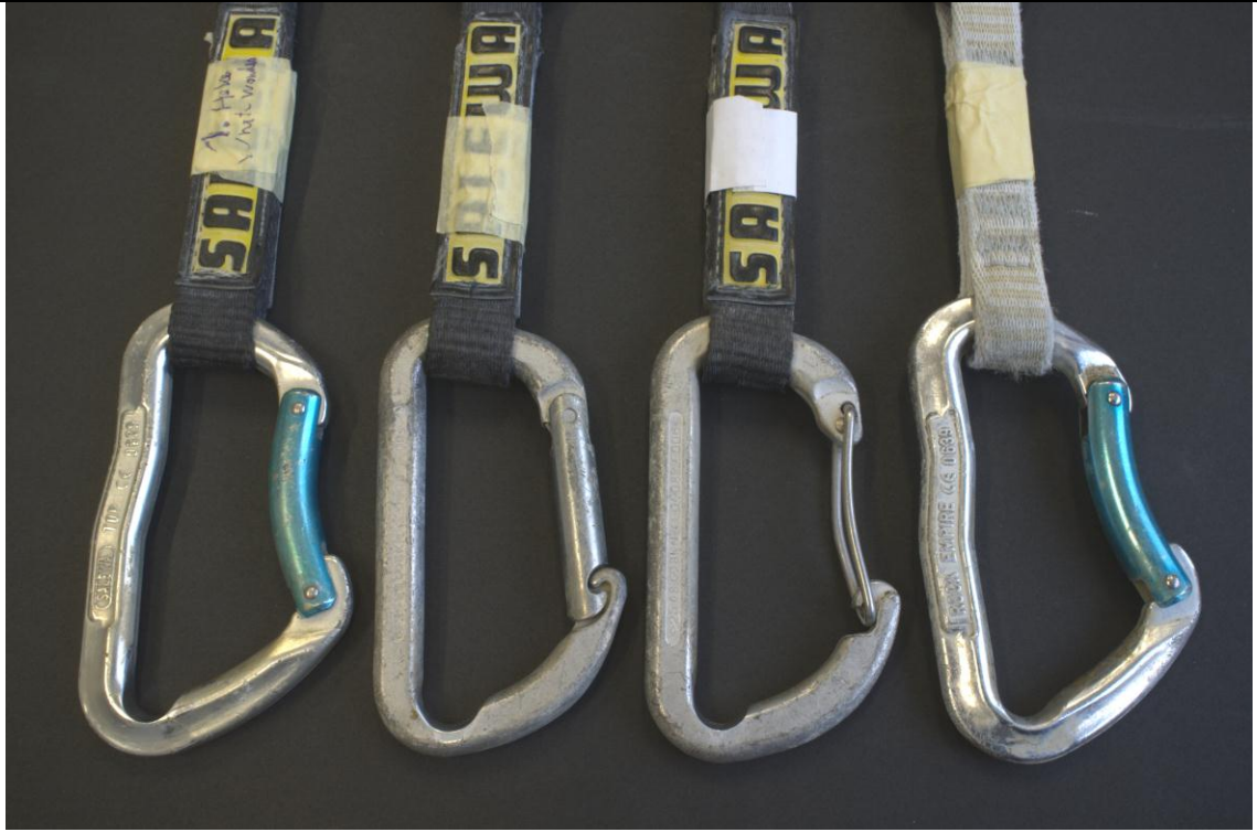
Figure 3 Fixed quick-draws from the Veil Falls sport crag (Klettergarten Schleier Wasserfall) in Tirol The abraded notches on fixed quick-draw carabiners—the various sharp edges are easily recognizable. Photos: Peter Plattner
